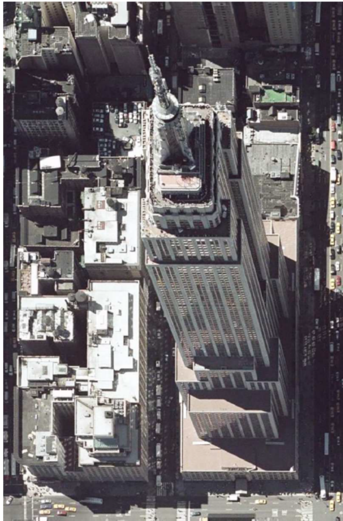
Figure 6-18: Tilt distortion is common on aerial and some satellite images, the result of perspective distortion when imaging the top and bottom of buildings, or any objects at different elevations.
