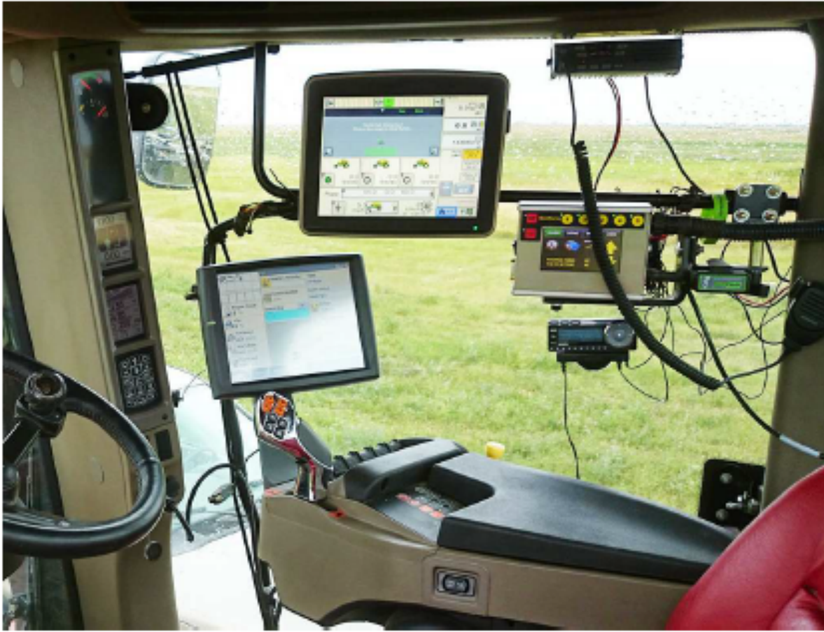
Figure 5-27: Line features may be field digitized via GPS, as in this example of a GIS/GPS system mounted in a tractor. Data display and digitizing software are used to record coordinates collected by a GPS receiver (above). An antenna placed on a pole or rack (right) reduces obstruction (courtesy Jake Leguee, left, and G. Johnson, Ducks Unlimited, right).
